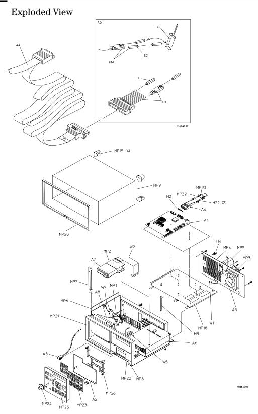
Exploded view of the 1664A logic analyzer.
